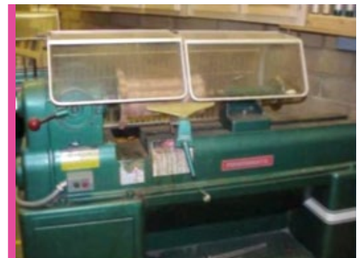
Wood lathe with guards in place.
